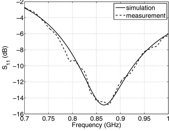
Fig. 7. Reflection coefficient of the bow-tie antenna.
