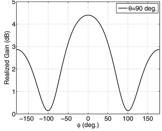
Fig. 9. The estimated rectenna realized gain. Only one antenna was radiated and the other, with the rectifier, acted as parasitic elements.
