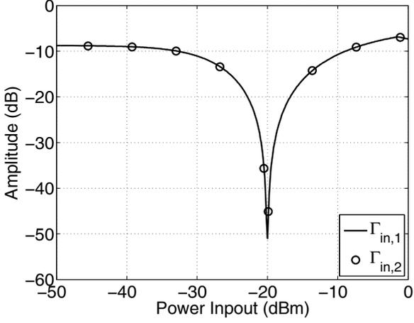
Fig. 3.  $\Gamma_{in}$  coefficient for two ports at 868 MHz.
