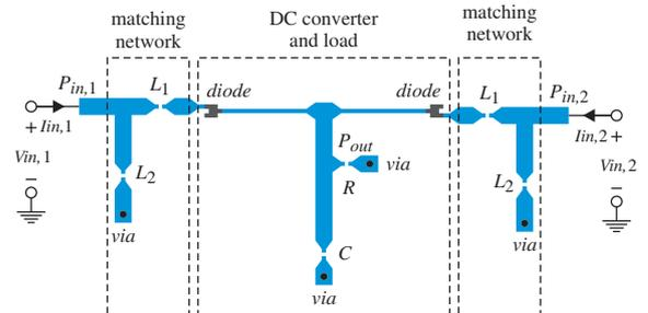
Fig. 1. Two-input microstrip rectifier-grid design (top layer).
