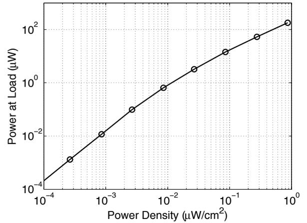
Fig. 14. The power at the load versus ambient power density.
