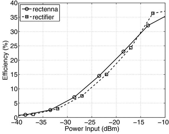
Fig. 11. Rectenna measured efficiency.
