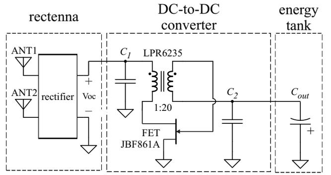
Fig. 15. Autonomous low-voltage and ultra-low power converter schematic with  $C_1 = C_2 = 1 \text{ nF}$  and  $C_{out} = 1 \text{ mF}$ .
