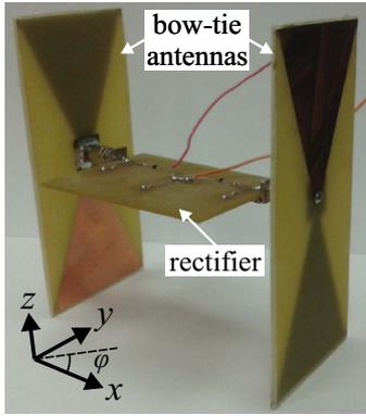
Fig. 8. The proposed rectenna-grid consisting of two identical bow-tie antennas.
