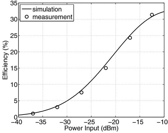
Fig. 4. Rectifier efficiency versus total power input.
