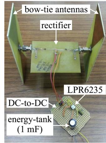
Fig. 16. The fabricated rectenna and the DC-to-DC converter.
