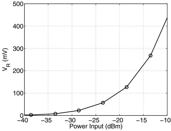
Fig. 12. Measured voltage across the 5 kOhm load.
