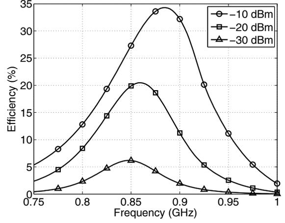
Fig. 5. Rectifier efficiency versus frequency for different power inputs.
