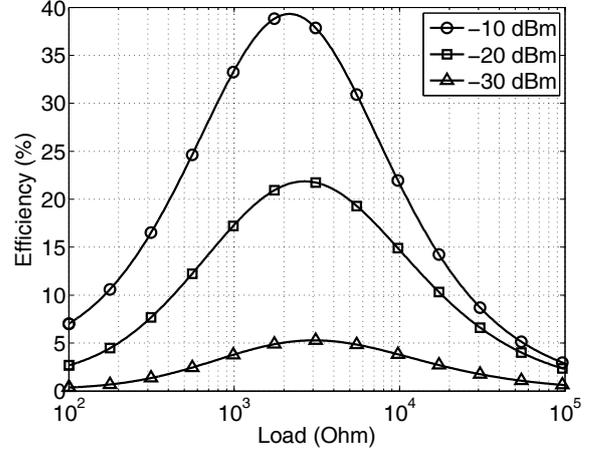
Fig. 6. Rectifier efficiency versus load for different power inputs.
