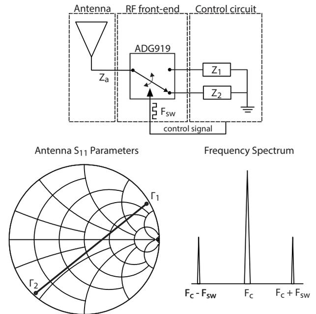
Fig. 1: Scatter radio communication principles: The low power RF switch “ADG919” alternates the termination loads ( $Z_1$  and  $Z_2$ ) of the antenna with frequency  $F_{sw}$ . When a carrier is equal with frequency  $F_c$ , two subcarriers appear, with frequencies  $F_c \pm F_{sw}$ .
