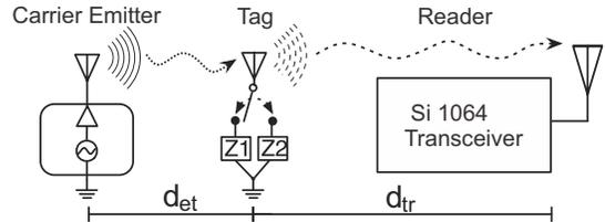
Fig. 2. Range measurements were implemented in the bistatic topology. Carrier emitter was far from the receiver.  $d_{et}$  denote the emitter-to-tag distance and  $d_{tr}$ , the tag-to-reader distance. Carrier emitter produces the signal which is modulated by sensor nodes and finally, the reflected signal is received by the reader.
