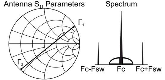
Fig. 1. FSK scatter radio communication principle: single, low-cost RF switch is utilized that alternates the antenna termination load between two values ( $Z_1$  and  $Z_2$ ) with switching frequency  $F_{sw}$ . Different antenna termination loads offer different reflection coefficients (left) that modulate a carrier signal with different amplitude and phase. For carrier frequency  $F_c$ , two subcarriers appear with frequencies  $F_c \pm F_{sw}$ .
