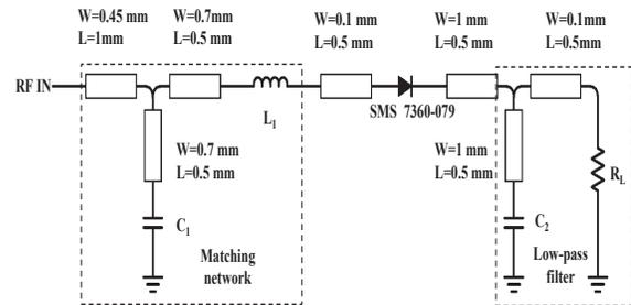
Fig. 3: Schematic of the designed rectifier circuit.
