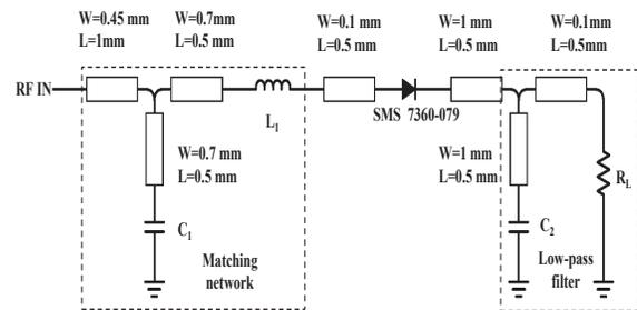
Fig. 3: Schematic of the designed rectifier circuit.
