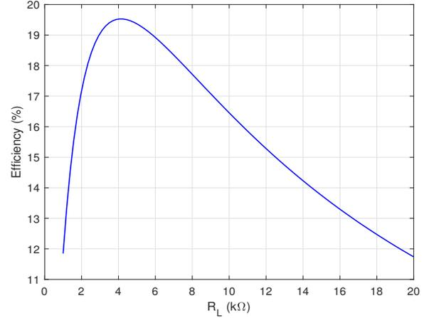
Fig. 6: Simulated rectifier efficiency vs. the output resistance ( $R_L$ ) at  $P_{in} = -20$  dBm.
