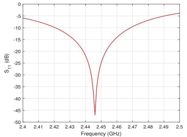
Fig. 8: Simulated reflection coefficient for the optimized layout vs. frequency at  $P_{in} = -20$  dBm.
