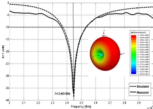
Fig. 2: Measured and simulated reflection coefficients versus frequency for the designed MIFA. Inset: plot of the 3D antenna radiation pattern
