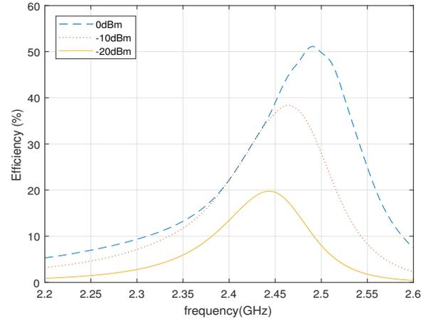
Fig. 7: Simulated rectifier efficiency vs. frequency at different power levels.
