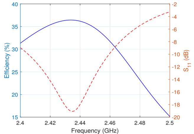
Fig. 4: Simulated rectifier efficiency and reflection coefficient vs. frequency.
