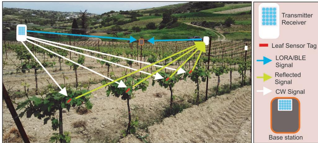
Figure 3.1: Agricultural backscatter communication setup in bistatic architecture. An emitter sends a pure carrier signal and a reader receives the modulated reflections of each tag. The tags could be embedded on leaf sensors for precise water stress monitoring.
