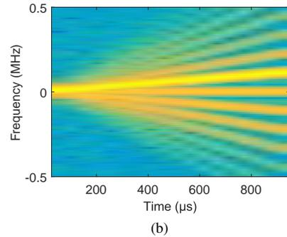
Fig. 6. Chirp based on one symbol from preamble of LoRa modulation with a SF of 7, with 125 kHz of bandwidth and time duration of 1 ms. a) Original chirp synthesized with our system. b) Obtained chirp from the measurement setup.
