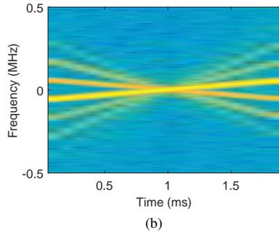
Fig. 4. Chirp with 125 kHz of bandwidth and time duration of 2 ms. a) Original chirp synthesized with our system. b) Obtained chirp from the measurement setup.
