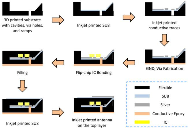
Fig. 2. Fabrication process for multilayer printing.
