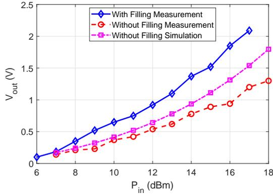
Fig. 6. Measured and simulated output voltage with respect to different input power at 26 GHz for the embedded energy harvester.
