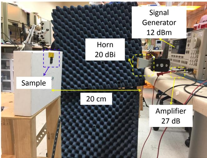
Fig. 10. Wireless performance evaluation for the system.
