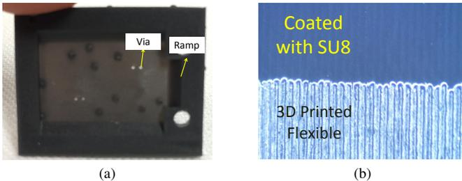
Fig. 3. (a) 3D printed substrate with cavity, ramps, and vias. (b) Substrate coated with SU8.
