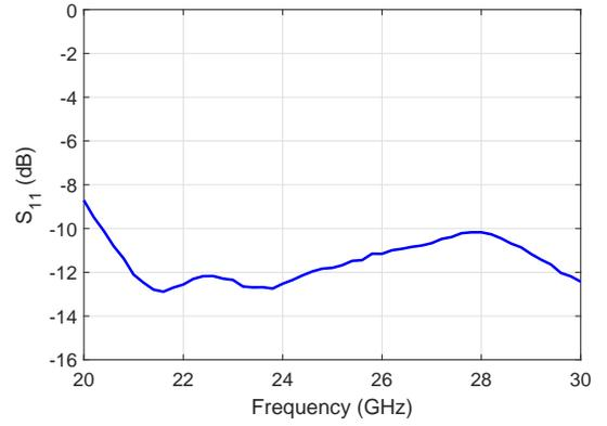
Fig. 8. Measured S11 for the antenna array.
