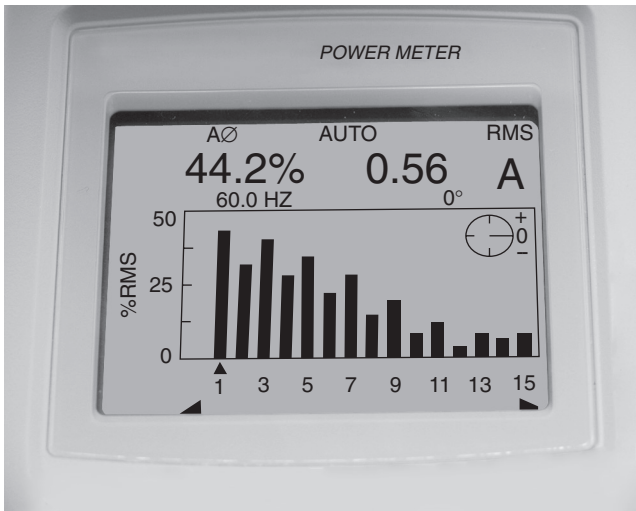
FIGURE 18-31. Harmonic current from of a small switching power supply, displayed on a harmonic meter.
