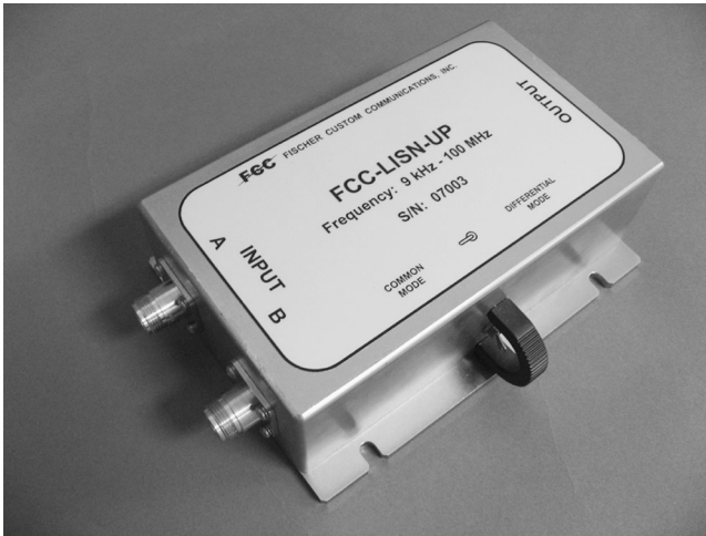
FIGURE 18-19. A commercial version of the combination differential- and common-mode rejection network used for conducted emission testing (courtesy of Fischer Custom Communications, Inc.).
