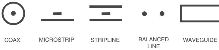
FIGURE 5-17. Some common transmission line geometries.
