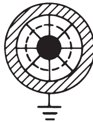
FIGURE 2-21. Fields around shielded conductor; shield grounded and carrying a current equal to the conductor current but in the opposite direction.
